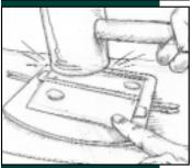
Repeat this process until 1<sup>st</sup> horizontal row is completed. Use a level to insure glass block is straight, plumb and level. Use shims under first row if necessary to adjust. Leave shims in until glass block wall is completed. Remove only after grout is applied and cured. Now is a good time to snap together the rest of the angle spacer halves. **Make sure they are fully snapped together by tapping with a rubber mallet. Angled spacersmust be fully compressed to ensure correct spacing.**
